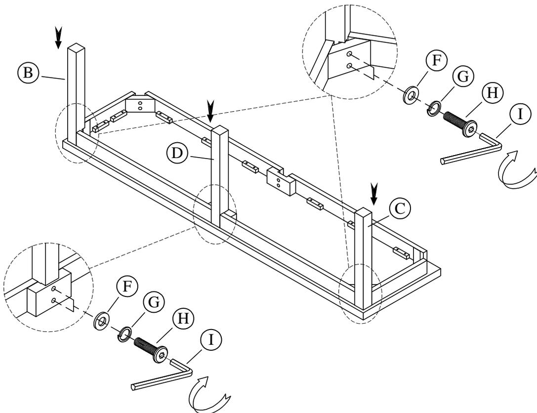
STEP 2: Do not fully tighten screws
