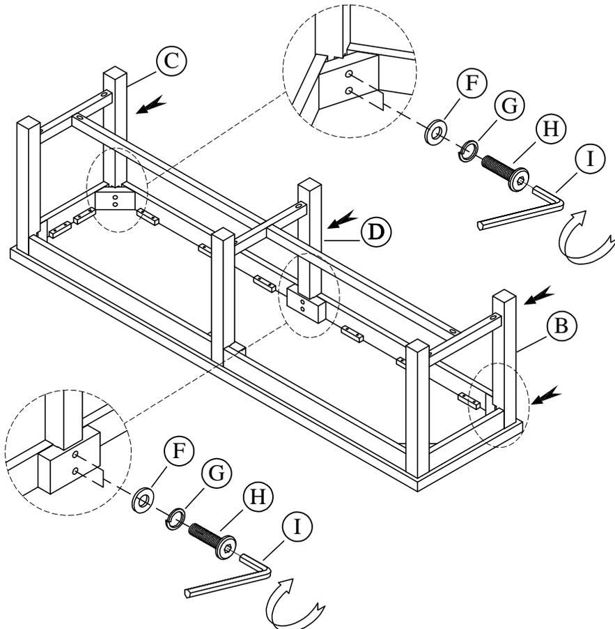
STEP 4: Using the Allen key and a Phillips head screw driver, tighten all bolts, then tighten all screws.
